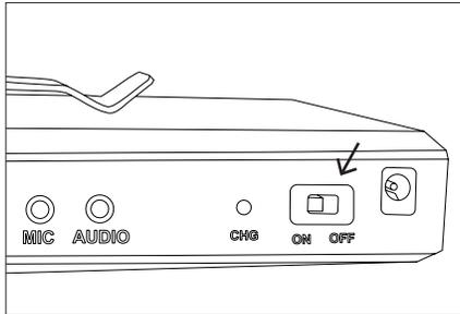
1. Turn on your Bolt 2.1/2.2 Transmitter using the ON/OFF switch found on the side of the unit.
