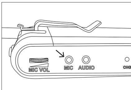
5. If using a mic, connect it to the Bolt 2.1/2.2's MIC input jack. **To enable the mic, press the button on the top of the transmitter.** The LED on top will turn red, indicating that the mic is on. Press the button again to mute the mic. The LED on top of the transmitter will turn off when the mic is muted.
