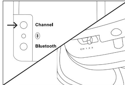
2. Using the CHANNEL button on your transmitter, choose channel 1, 2, or 3 to broadcast an audio signal. Make sure that your GLO 2 headphones are set to receive the same channel. The headphones' power and channel switches are located on the left ear.
