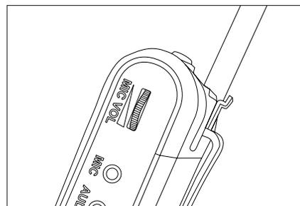
6. Control the mic's volume using the MIC VOL dial on the side of the transmitter.
