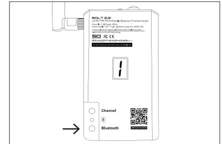
4. Put the transmitter into pairing mode by holding down the BLUETOOTH button until the LED flashes **RED AND BLUE**. The transmitter will appear in your device's Bluetooth menu as "Bolt 2.2" or "TX60RF." The LED will turn solid blue to indicate a successful Bluetooth connection. Hold down the BLUETOOTH button again to disable the connection. Enabling the Bluetooth connection automatically mutes the AUDIO input jack.
