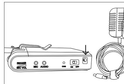
7. To recharge your Bolt 2.1/ 2.2's battery, connect the AC power adapter to wall power. The CHG LED will turn from red to green when the transmitter is fully charged.
