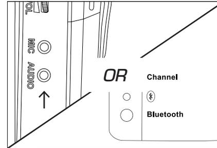
3. If using a playback device such as a phone, laptop, or mixer, connect it to your Bolt 2.1/2.2 using either the stereo AUDIO input jack or the Bluetooth connection. Set your playback device's volume to about 90%. **Warning: do not plug any device except for a microphone into the MIC jack. Doing so may cause distortion and can damage your transmitter.**
